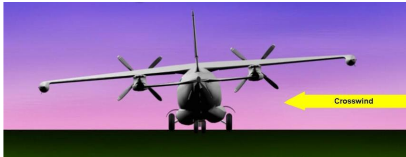
Fig.1 – Downwind Lean Caused by Crosswind
